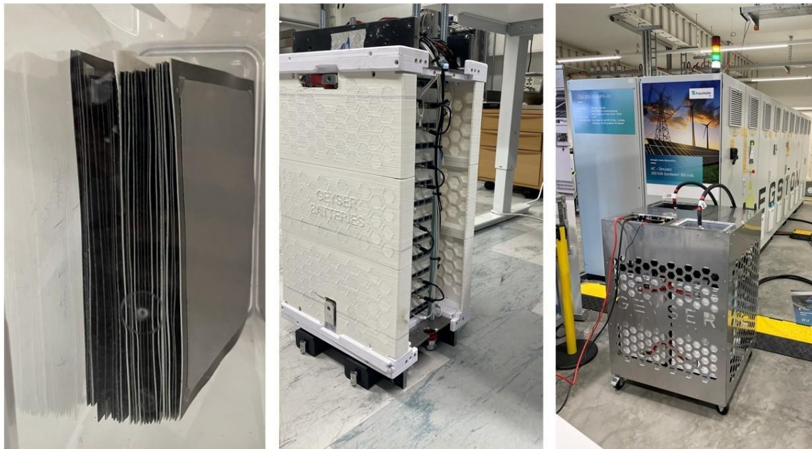
Figure 1.1 – (Left) Geyser Batteries Cells. (Middle) Vertical Sub-units for Modular Assembly. (Right) Assembled Module being Tested at Fraunhofer IEE.
